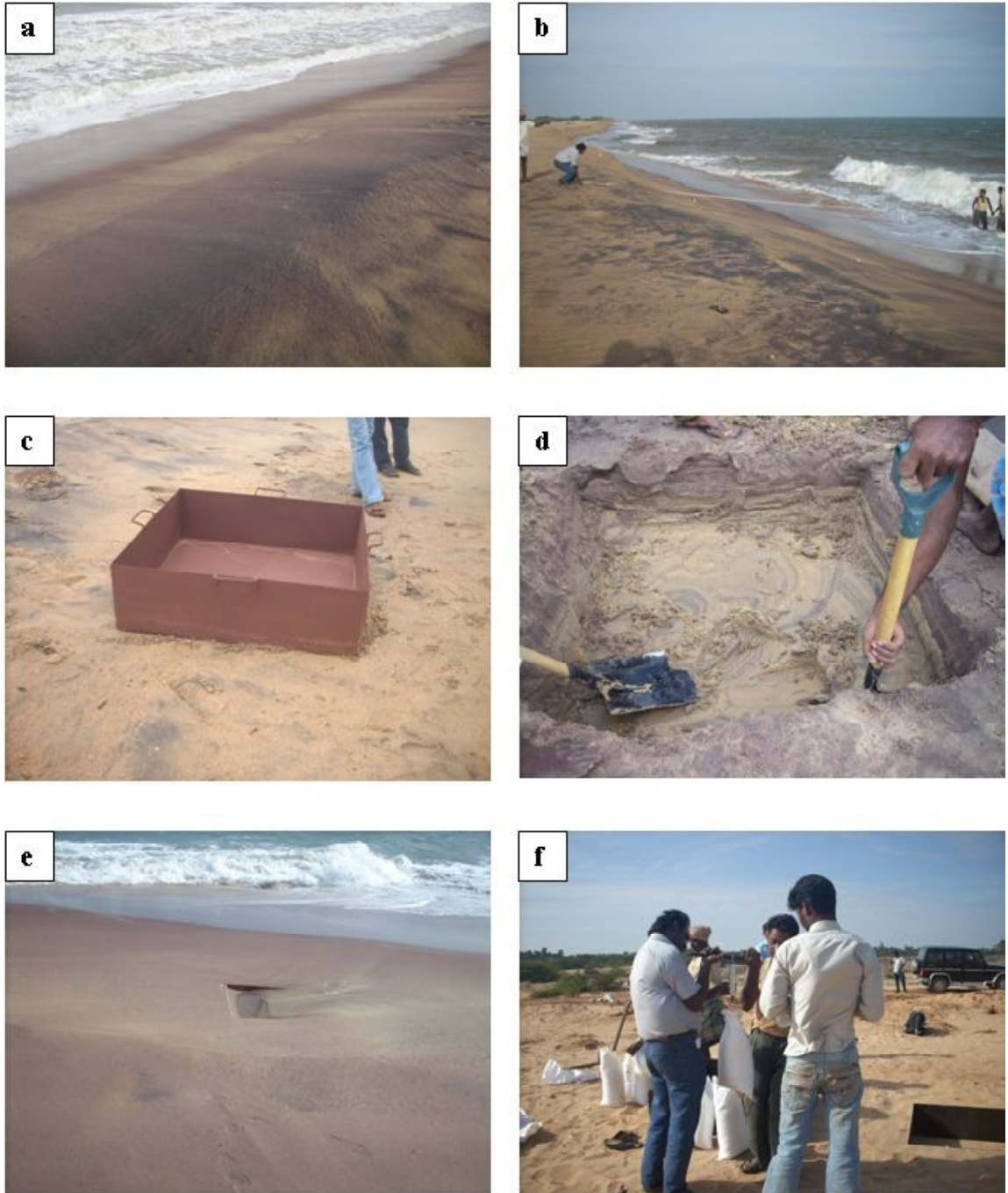
Fig. 3. Photographs showing a) beach placer deposit at Vaippar, b) measurement of zones c)steel box for replenishment study, d) pit for placing steel box, e) box placed in the tidal zone f) weighing of collected mineral sand
